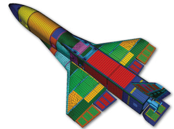
Finite element analysis model of the X-34
