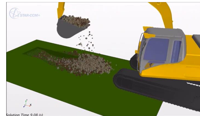
Excavation of rocks using DEM
