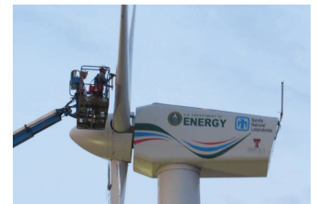
Full turbines were tested to obtain frequencies for model comparison
