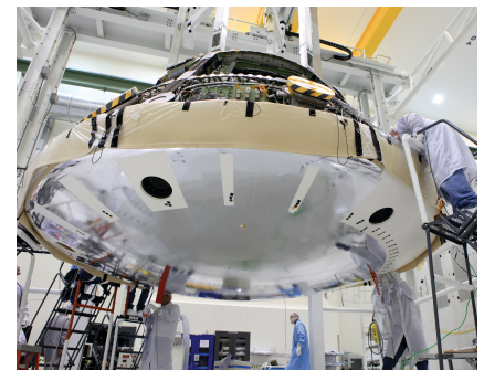
Underside view of Orion's heatshield, the largest heatshield ever built Image courtesy of NASA
