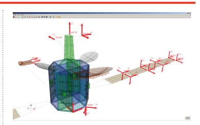
Visualize coordinate trace locations and orientation on your FEM using VTK with IMAT+FEA.
