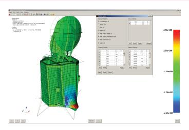
Display stress results on a deformed mesh, and selectively display FEM entities by type, group, or both with IMAT+FEA.
