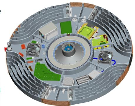
▲ CAD geometry of SATCOM electronics compartment
