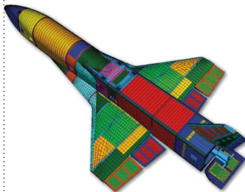
▲ Finite element analysis model of the X-34
