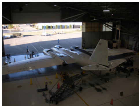
▲ WB-57F undergoing ground vibration testing
