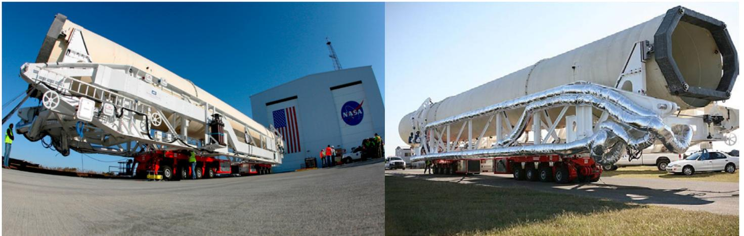
▲ Figure 6: Completed TEL transporting a payload from integration facility to launch pad.
