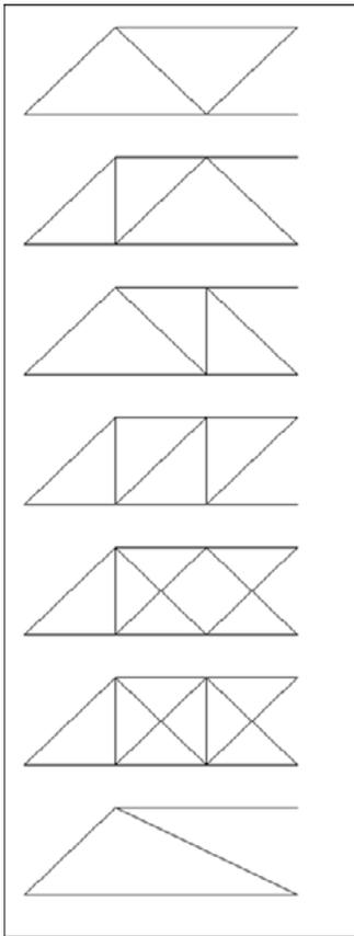
▲ Figure 3: Truss systems considered for strongback design.
