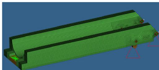
▲ Figure 1: Meshed design space for TEL strongback in preparation for topological optimization.
