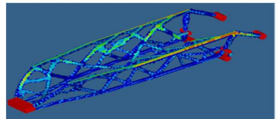
▲ Figure 2: Optimization results showing regions of critical structure for primary load case.
