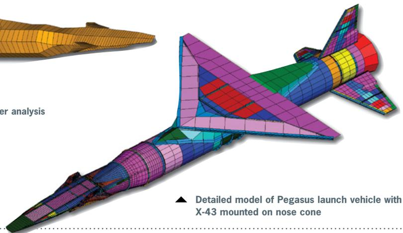
▲ Detailed model of Pegasus launch vehicle with X-43 mounted on nose cone
